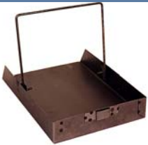
A035. RAYBURN SUPREME ASHPAN W297 X H65 X D382 (TAPER 297) mm
